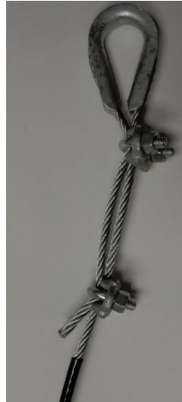
Figure 6 – Thimble, Rope and Rope Clips Assembly
