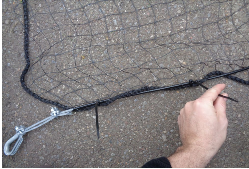
Figure 7 - Wire Rope to Bottom of Net Assembly
