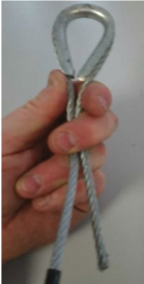
Figure 5 – Thimble and Rope Assembly
