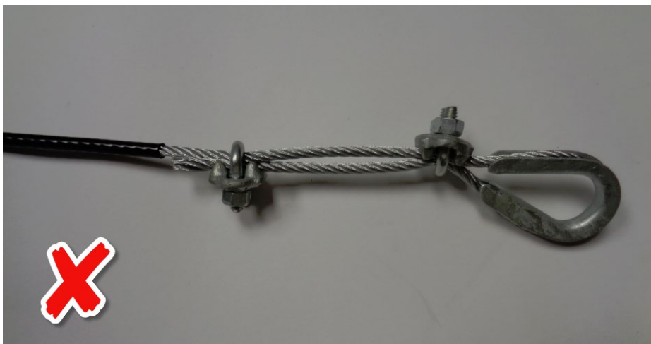
Figure 4 - Wire Rope, Thimble and Rope Clips Assembly
