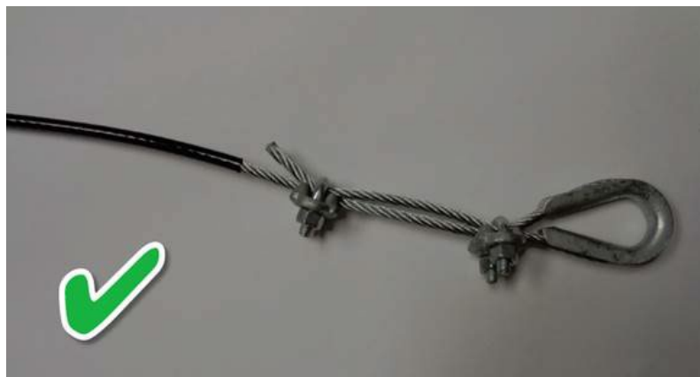
Figure 6 - Wire Cable Loop at End of Net
