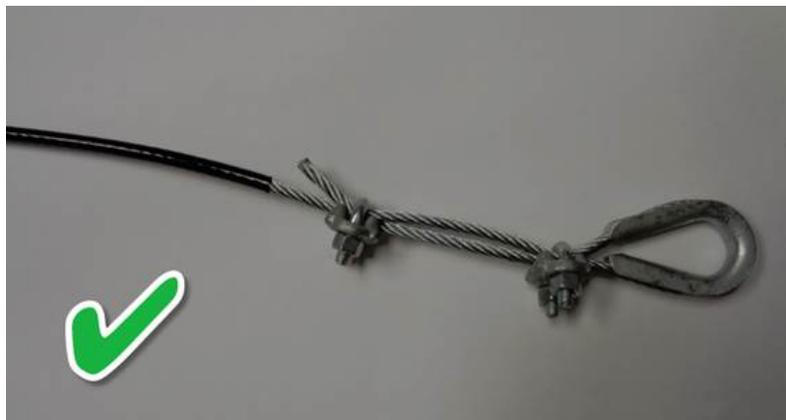
**Figure 6 - Wire Cable Loop at End of Net**
