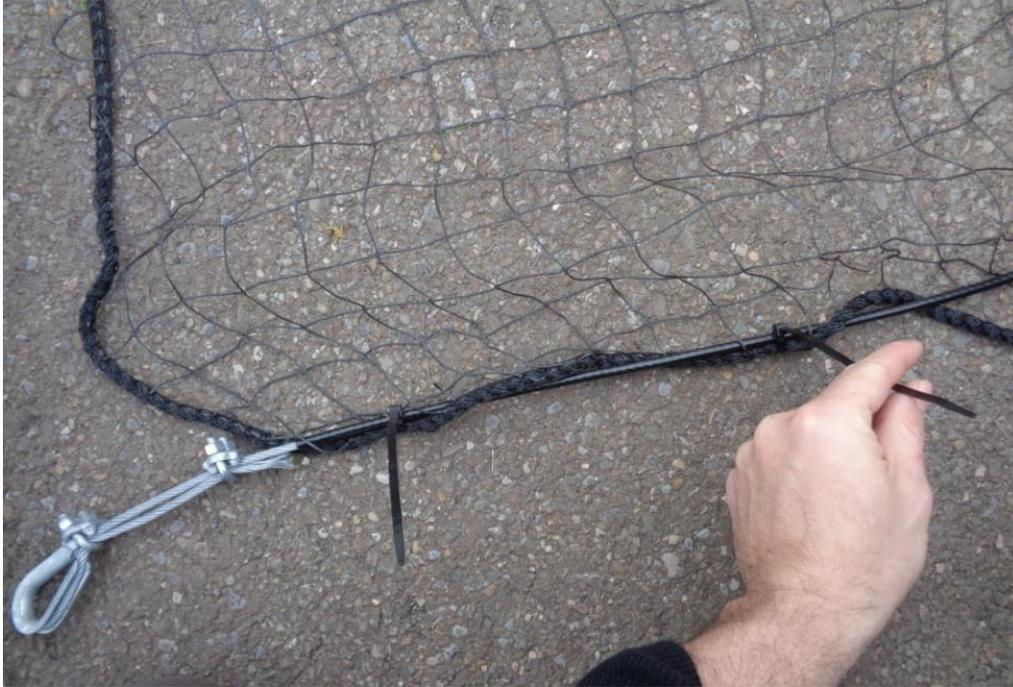
**Figure 8 - Wire Rope to Bottom of Net Assembly**
