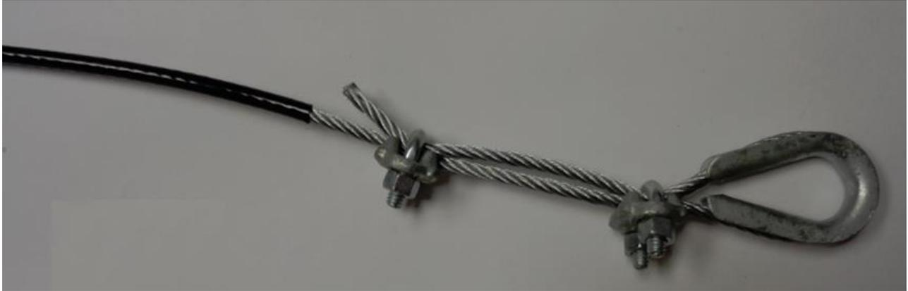
**Figure 7 – Thimble, Rope and Rope Clips Assembly**
